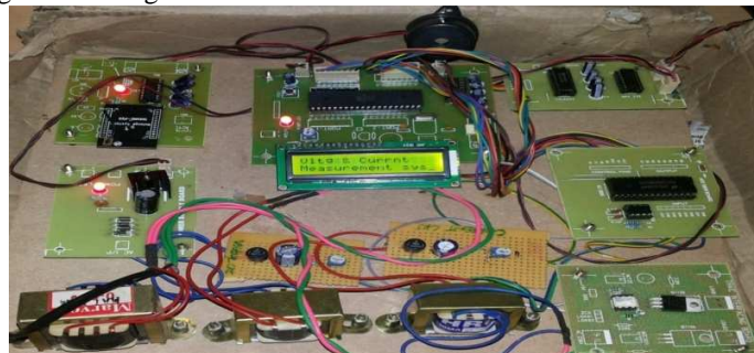
Fig.9: Ready to Work for Voltage and Current Measurement System.
